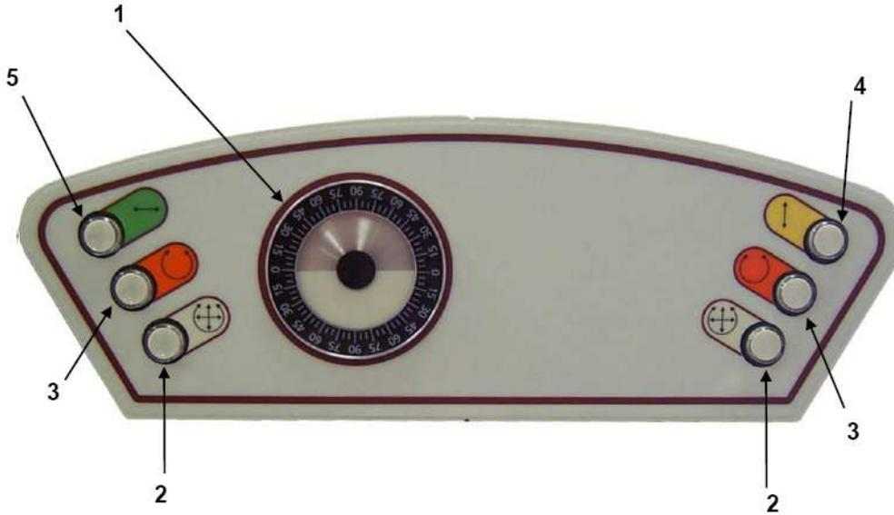
**Pos. 1** -> Angle indicator, indicates angle of the X-ray tube assembly.
