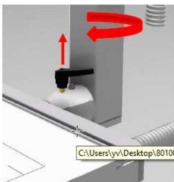
By lifting (pulling) the lever the serration is released and the lever can be put into the most favourable locking or unlocking position. When "letting go" the lever, it will catch again.
