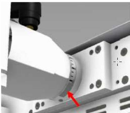
The rotation movements of the arm gives you the possibility to set an angle for oblique projections or even to rotate by 90° in order to perform e. g. a radiography of the foot on the floor.
