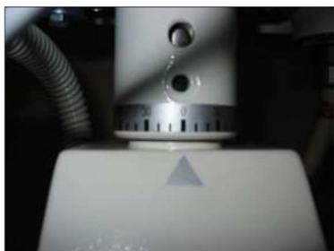
The values on the rotation dial indicate the brake points. Set the 0° initial position using the collimator and docking station mark.
