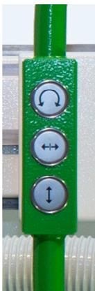
The universal support is used to set the position of the X-ray source (X-ray tube) and the X-raying unit (flat panel detector in the docking station), or to set them in another position such as the floor, wall or table, as required.
