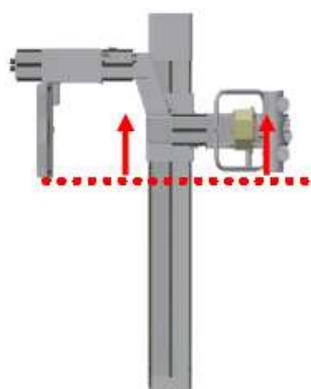
The vertical carriage with the transversal arm is kept in balance by a spring inside the wall column. If the carriage is fixed at the highest position, the spring is only under light stress. If, however, the vertical carriage is fixed at the lowest position, the spring is under maximum stress.
