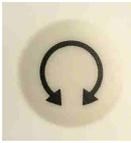
This button releases the cross arm brake, allowing the cross arm to rotate. The rotation dial displays the degree of rotation in relation to the initial horizontal position.
