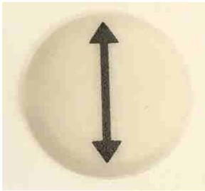
Pressing this button releases the brake of the vertical carriage. The vertical carriage can be moved up and down by hand while pressing the button.
