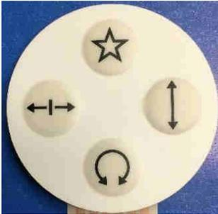
The universal support is used to set the position of the X-ray source (X-ray tube) and the image receptor (film cassette/flat panel detector) in the Bucky or any other position such as the floor, patient table, etc. There are three different axes. Pressing a button releases an electromagnetic brake lock in each axis. These buttons are located on the cross arm control unit.
