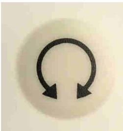
This button releases the cross arm brake, allowing the cross arm to rotate. The rotation dial displays the degree of rotation in relation to the initial horizontal position.
