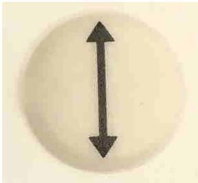
Pressing this button releases the brake of the vertical carriage. The vertical carriage can be moved up and down by hand while pressing the button.
