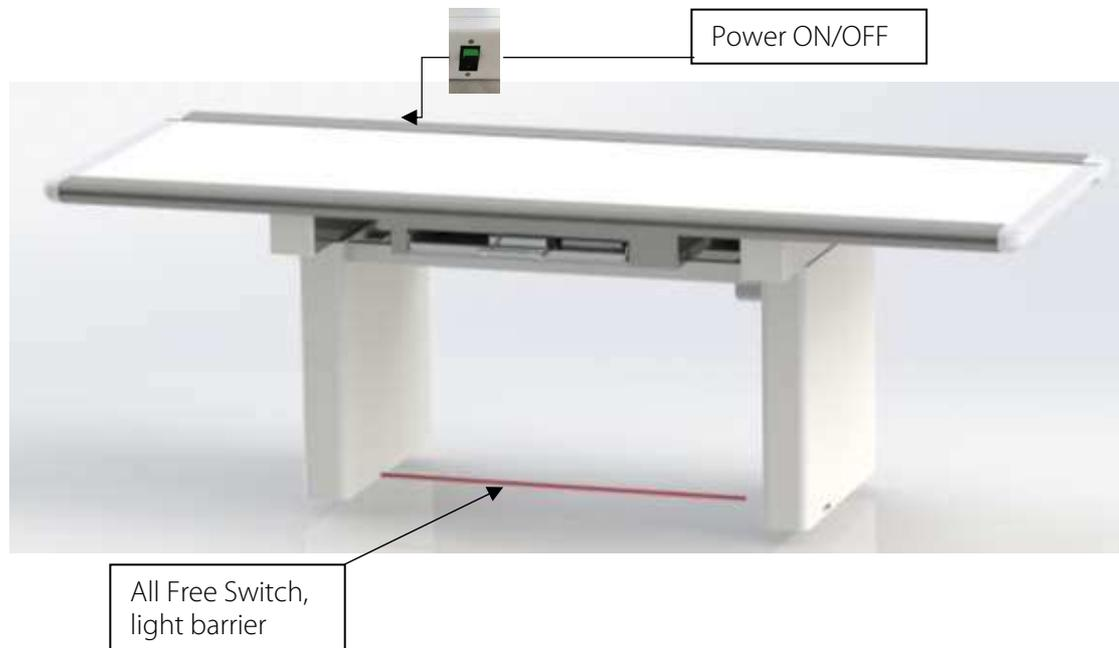
The red line in the figure is the "ALL-FREE" switch. By bringing a foot or any object in this area, the "ALL-FREE" switch will be activated. With the switch checked, it is available to move the table top in any direction.
