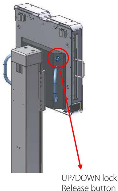
For vertical movement of Bucky, it is available to move either up or down the Bucky manually while holding the UP/DOWN button as the figure. Detailed information please find in the enclosed User Manual of the PROGNOST C.
