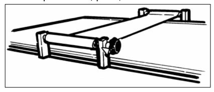
The compression band (7) is inserted into the PA profile rails of the table top. The transparent band-shaped compressorium can be used to apply pressure to the body part to be examined or to hold the body in rest position. The tensile force is adjusted self-locking.
