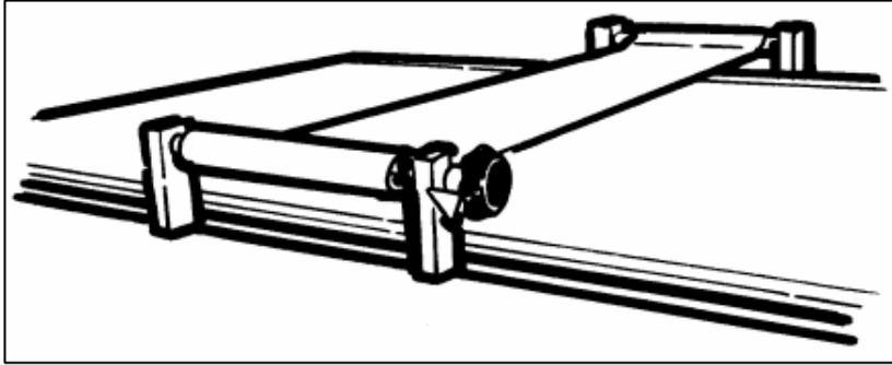
The compression band (7) is inserted into the PA profile rails of the tabletop. The transparent band-shaped compressorium can be used to apply pressure to the body part to be examined or to hold the body in rest position. The tensile force is adjusted self-locking.
