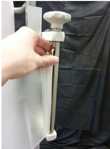
Step 4: Hold the band and turn the hand wheel to fasten the compression band.
