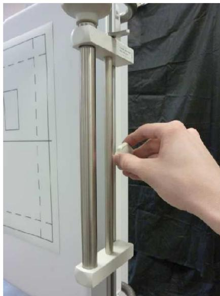
Step 2: Insert the fixed stretching roller into the support rail on the left side and fix it at the same height as the roller on the right rail. Insert the compression band and pull it around the stretching roller.
