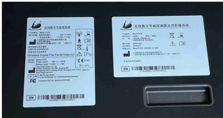
The type labels are located on the underside of the detector.
