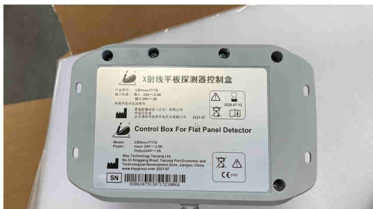
The type labels are located on the underside of the control box.
