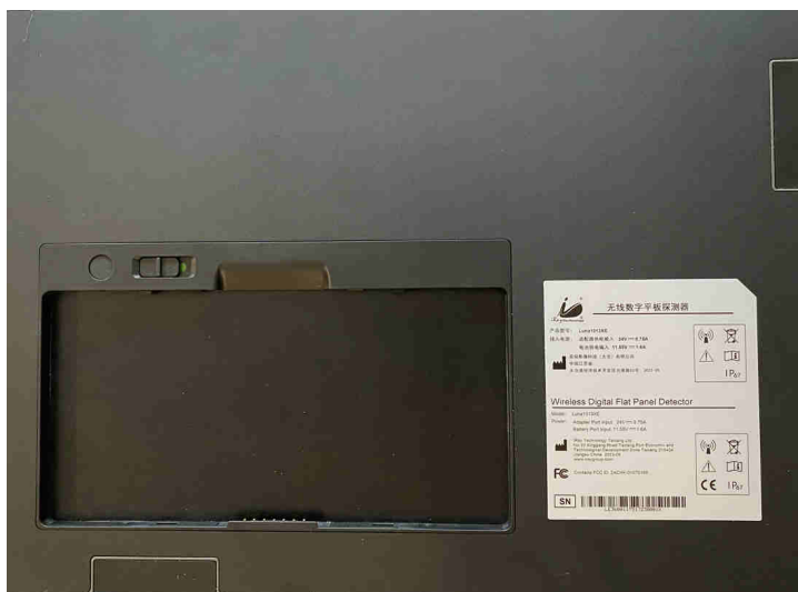
The type labels are located on the underside of the detector.
