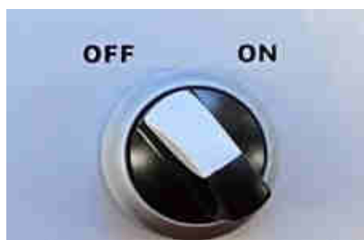
Fig. 3.1c Power Box Switch
