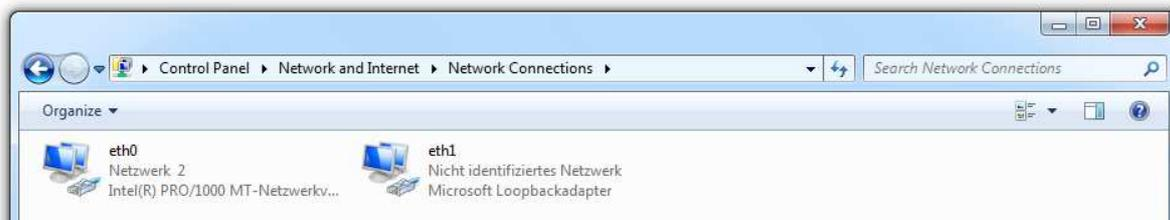
Select the network adapter where the MP-Box is connected with the right mouse button and press "PROPERTIES". Select the list entry "INTERNET PROTOCOL VERSION 4 (TCP/IPv4)" and press "PROPERTIES". Set up the IP address 192.168.0.10. Change the subnet mask to 255.255.255.0.
