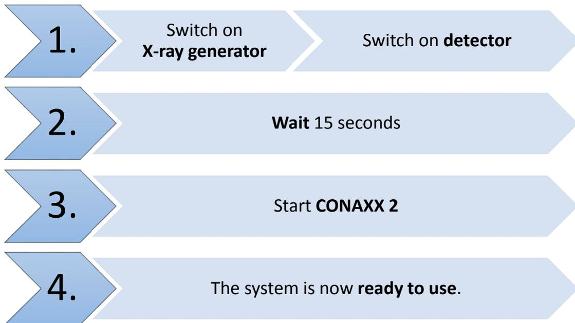
If CONAXX 2 cannot connect to the modality or generator after launching the program there will appear an error message. In this case, CONAXX 2 has to be restarted to initiate a new connection. Further hints you can find in the indicated error message.
